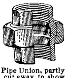
Pipe Union, partly cut away to show construction.
