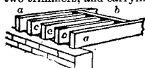
Timbers with Header. a a Trimmers; b Header; c c c Tailpieces or Tail Beams.
